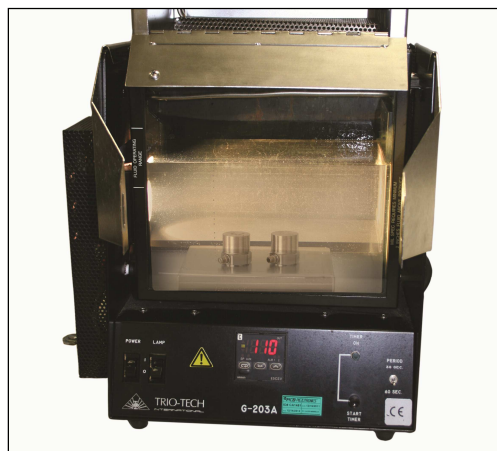
Figure 8: Gross Leak Test Apparatus
