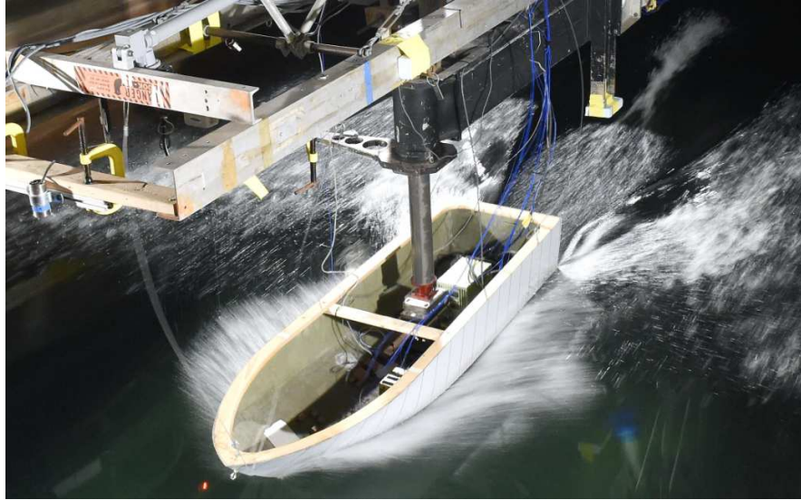
Figure 1: Typical Open Tunnel Water Test of Ship Hull Photo by: John F. Williams
