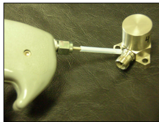
Figure 9: Leak Detection ‘Sniff’ Test on Weld Joint of a Hermetic Connector
