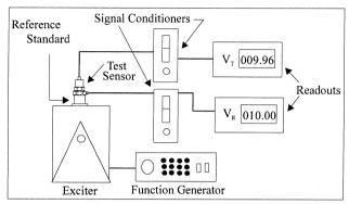
Figure 10. Typical Back-to-Back Calibration System
