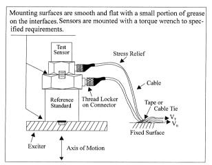
Figure 12. Typical Calibration Set-Up
