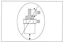
Figure 15. Mounting Triaxial Sensors (Incorrect)
