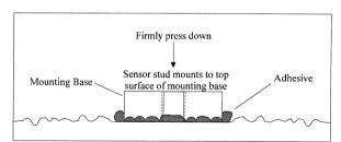
Figure 4. Mounting Base: Adhesive Installation
