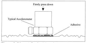
Figure 5. Direct Adhesive Mounting
