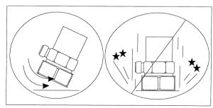
Figure 7. Magnet Mounting
