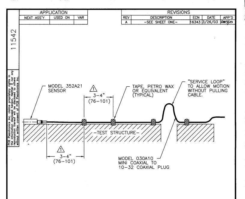
2.) TO AVOID UNNECESSARY DAMAGE TO THE SENSOR AND/OR CABLE, USE THE SUPPLIED REMOVAL TOOL (MODEL 039A27). A QUICK TWISTING MOTION WILL FREE THE SENSOR FROM THE TEST STRUCTURE.
