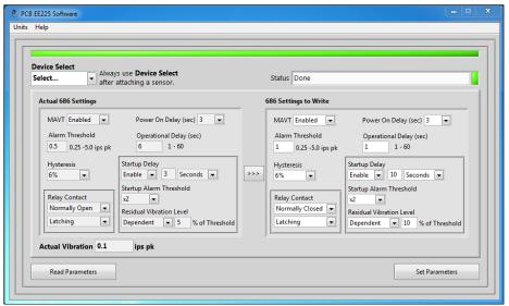
Figure 11 - Typical Smart Switch Screen After Successful Parameter Read
